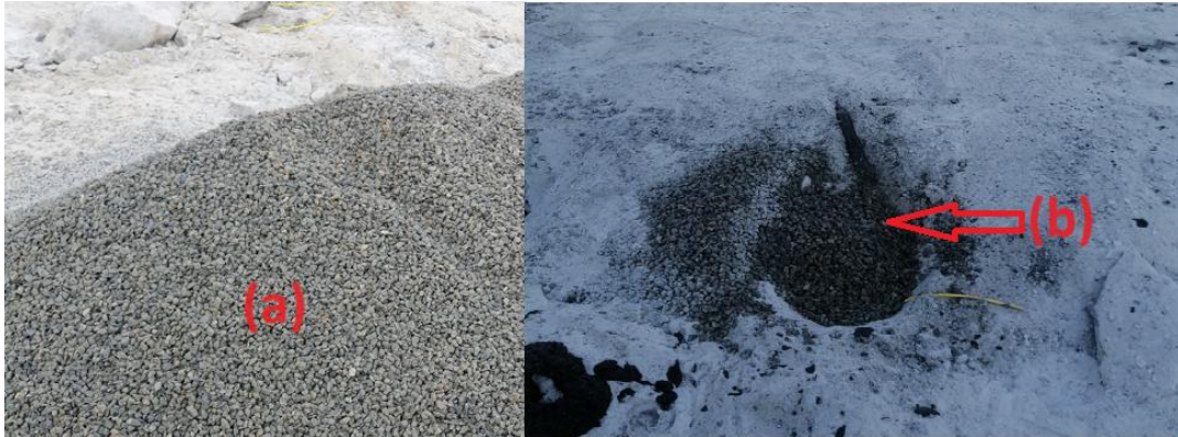
Figure 2.11: (a) Crushed aggregates; (b) Blasthole filled with crushed aggregates (Own picture taken by the author at Quarry TM)
