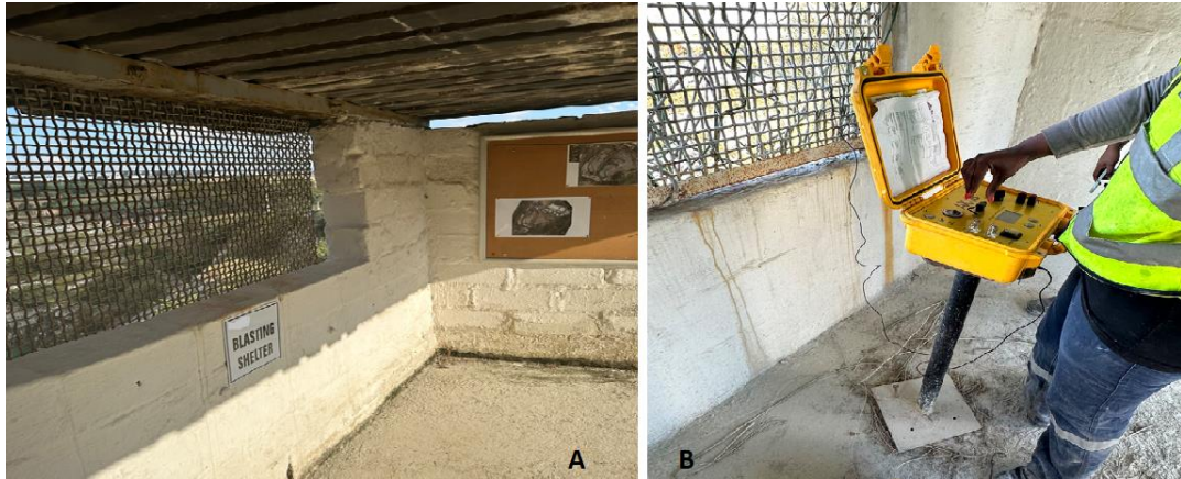
Figure 3.27: (A) Blasting shelter for mine personnel to gather and observe the blast, (B) Controller blasting box is set up in the blasting shelter (Source: Author's picture)
