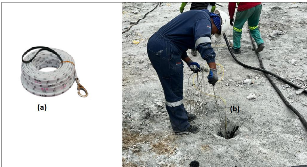
Figure 3.14: (a) Example of a typical measuring tape (Source: Better Blasting, 2021) and (b) Measuring of blasthole stemming length with measuring tape (Source: Author's picture)
