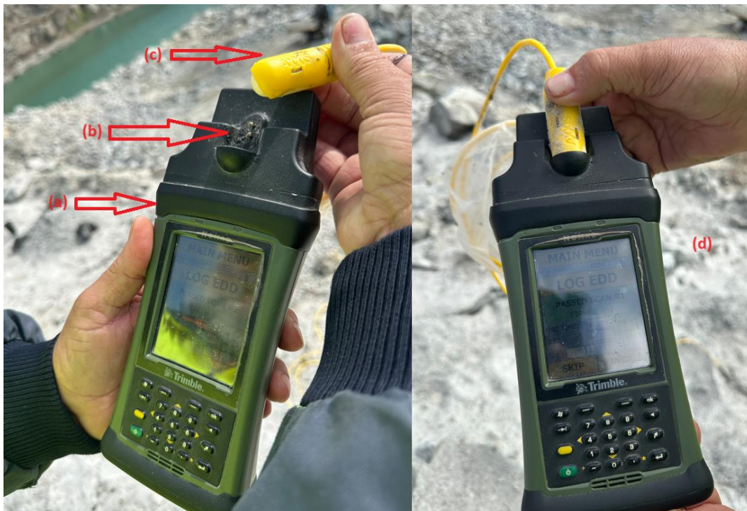
Figure 3.21: (a) AXXIS™ titanium logger, (b) slot where the detonator is to be inserted, (c) detonator, and (d) illustration of how the scanning of detonators is done (Source: Author's picture)
