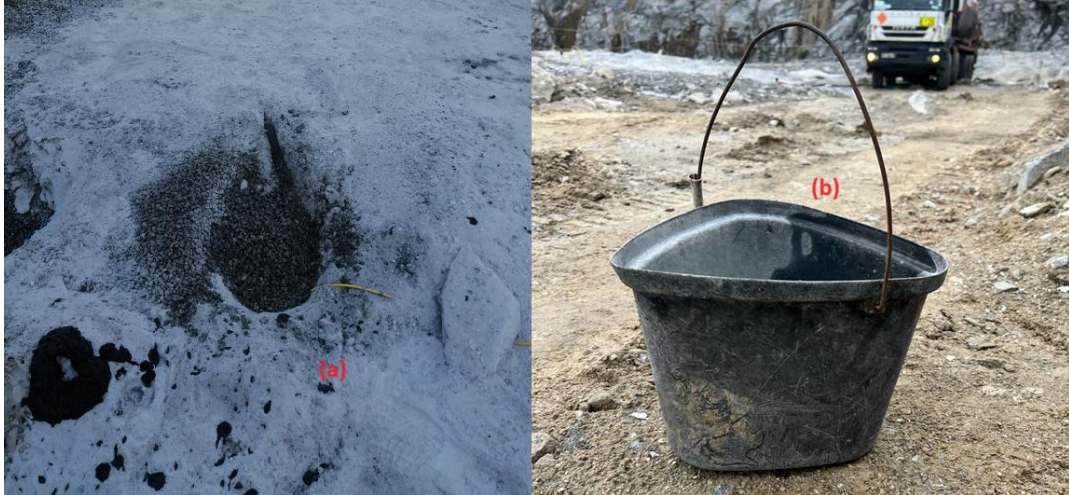
Figure 3.19: (a) Stemming of blastholes with crushed aggregates, (b) Buckets used to stem holes (Source: Author's picture)
