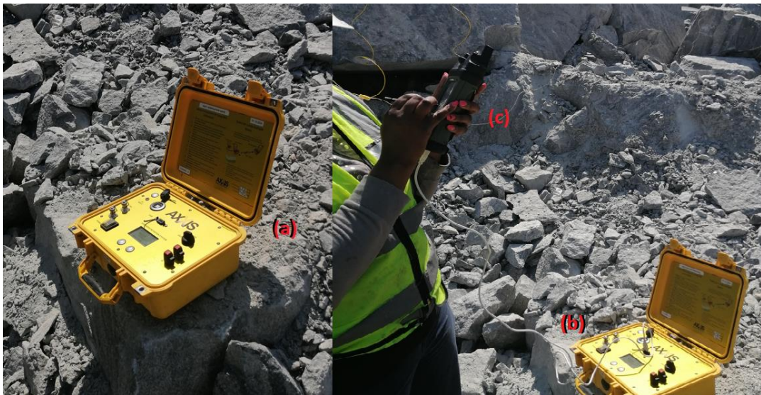
Figure 3.23: (a) AXXIS™ titanium blasting box on site, (b) Blasting box connected to a logger, and (c) Logger transferring information to the blasting box (Source: Author's picture)
