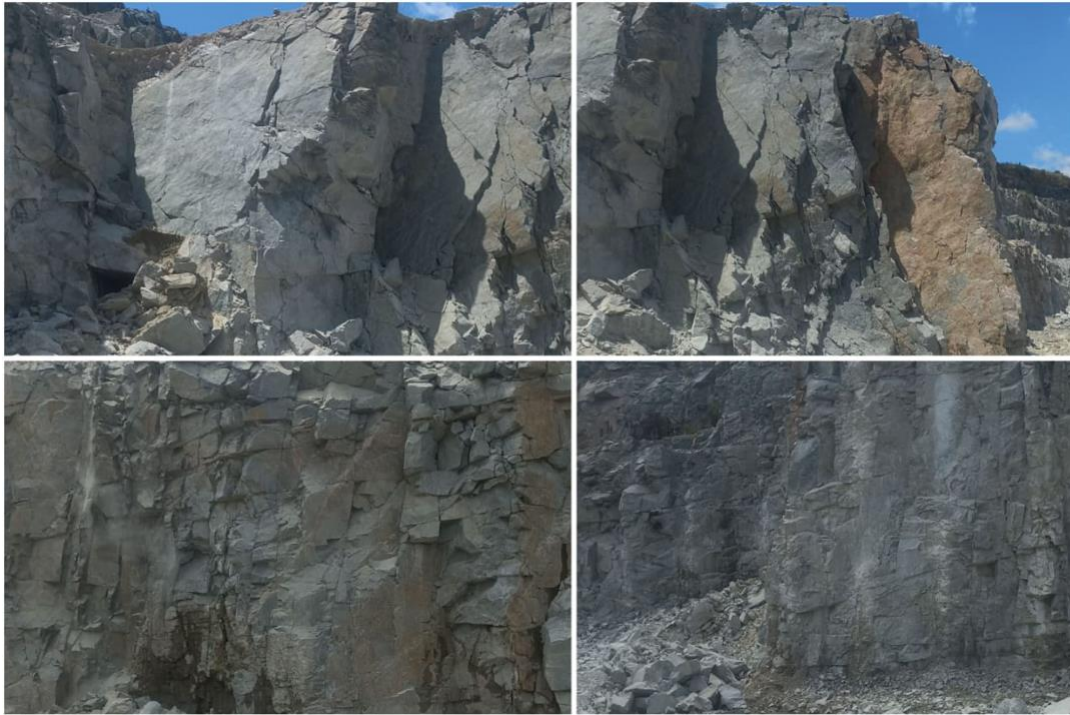
Figure 5.1: Geological discontinuities present within the rock mass – Field observation by the author at Quarry TM
