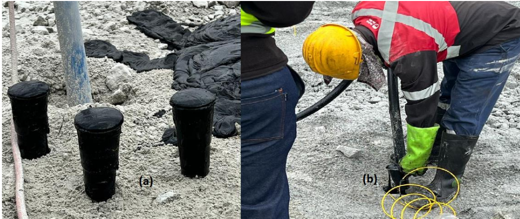
Figure 3.11: (a) Observing of gassing of the explosives inside the 400 g cups and (b) Filling the cups with the emulsion explosive (Source: Author's picture)
