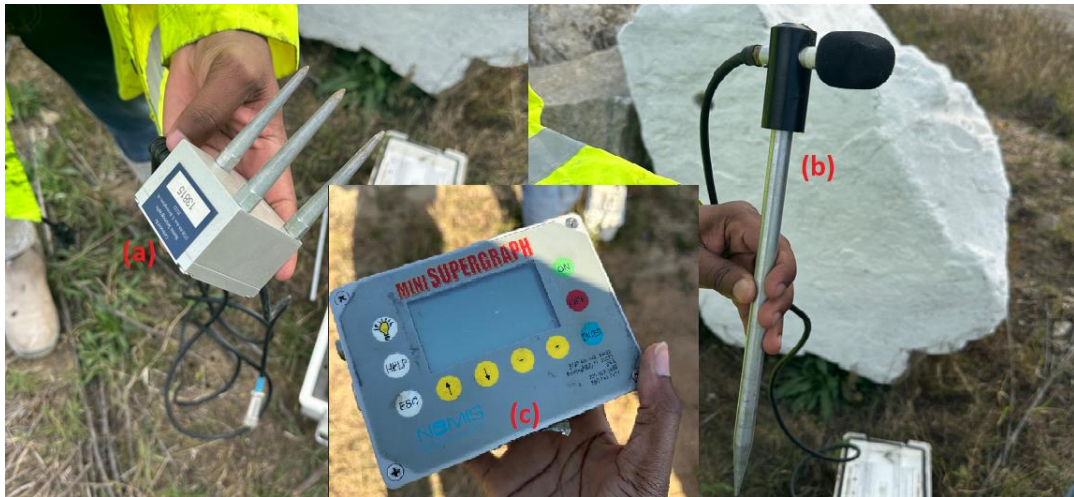
Figure 3.25: (a) Geophone, (b) Air overpressure transducer, and (c) Control unit (Source: Author's picture)
