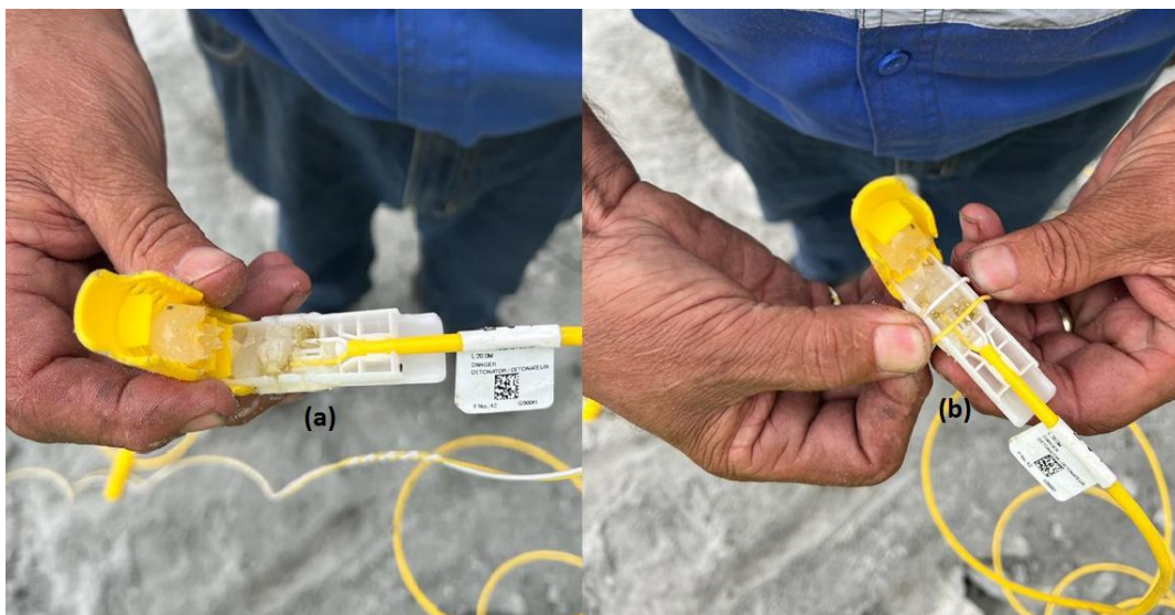
Figure 3.9: Detonator cord attached to a colour-coded connector clip (Source: Author's picture)
