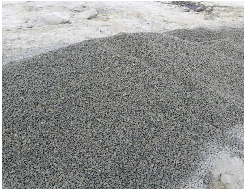
Figure 3.18: Crushed aggregates used for the stemming of blastholes (Source: Author's picture)
