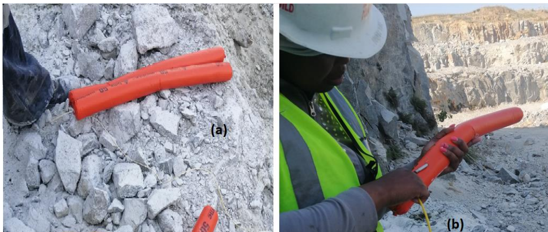
Figure 3.13: (a) Mega-mite 50 x 580 cartridges, and (b) Charging of 50 x 580 cartridge explosives with a detonator (Source: Author's pictures)
