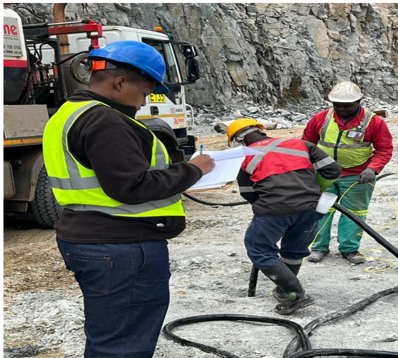
Figure 3.10: Charging of holes with emulsion explosives (Source: Author's picture)
