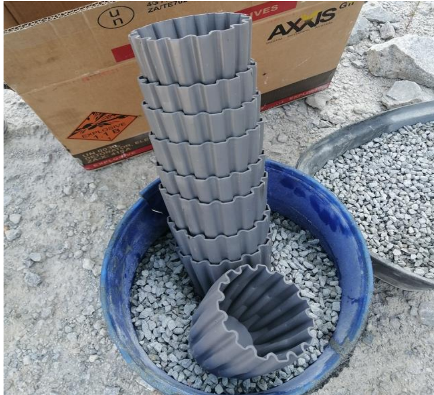
Figure 3.16: Varistem® stemming plugs of diameter 102 mm (Source: Author's picture)
