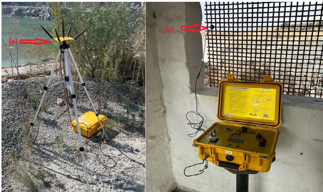
Figure 3.24: (a) Receiving antenna connected to a blasting box on site, and (b) Transmitting antenna connected to a blasting box in the blasting shelter (Source: Author's picture)
