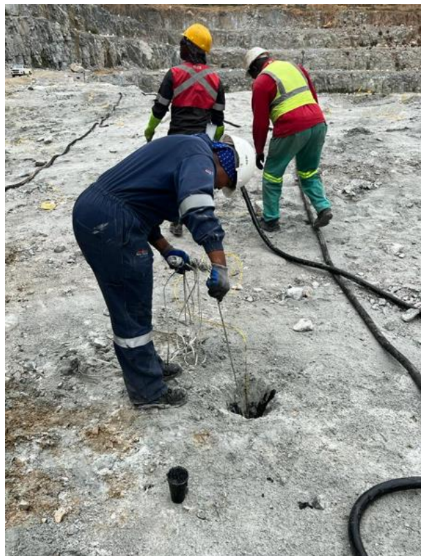
Figure 3.7: Measuring of drilled blastholes (Source: Author's picture)
