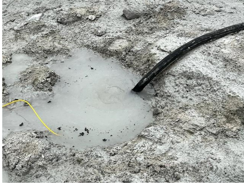
Figure 3.12: Displacement of water from the blasthole during charging (Source: Author's picture)
