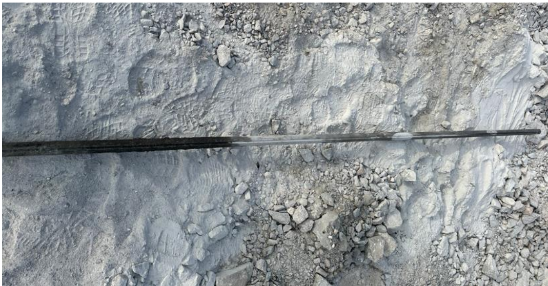
Figure 3.20: Tamping rod used to tamp the aggregates during stemming (Source: Author's picture)
