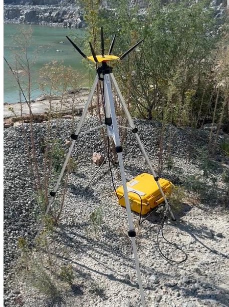
Figure 3.21: The AXXIS Titanium long-range electromagnetic transmitter plate antenna (Source: Photo taken on site)
