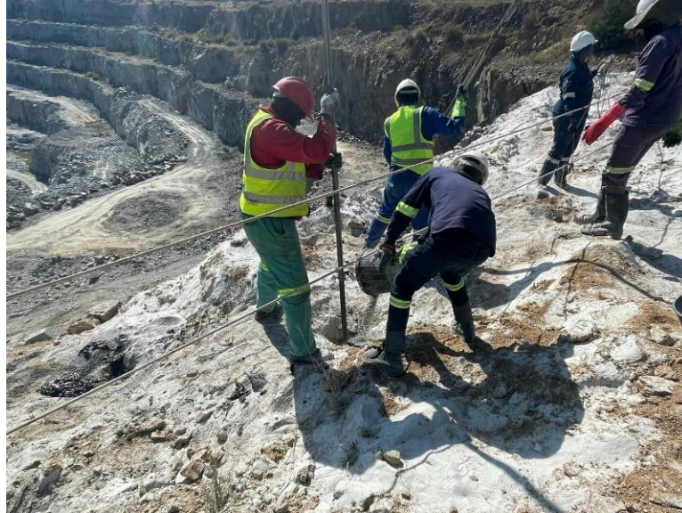
Figure 3.14: Tamping of stemming material (Source: Photo taken on site)
