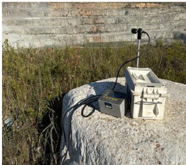
Figure 3.22: NOMIS Mini Supergraph seismograph (Source: Photo taken on site)
