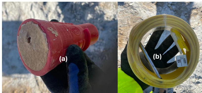
Figure 3.3: (a) C400 Trojan boosters and (b) AXXIS Titanium electronic delay detonator (Source: Photo taken on site)
