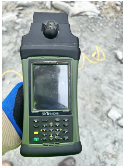
Figure 3.16: The logger used to program the timing of the detonators on site (Source: Photo taken on site)
