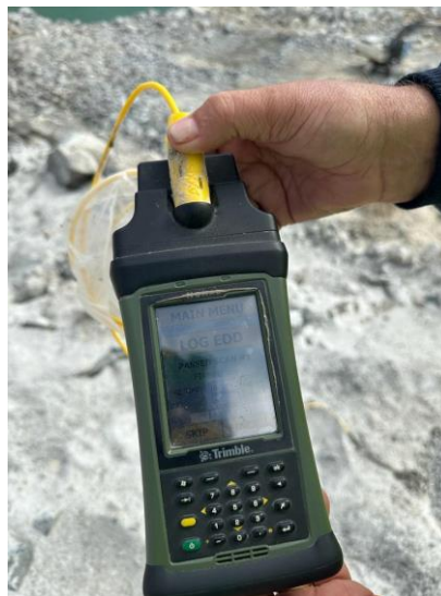
Figure 3.17: Illustration of how the connector of the electronic detonator is scanned (Source: Photo taken on site)
