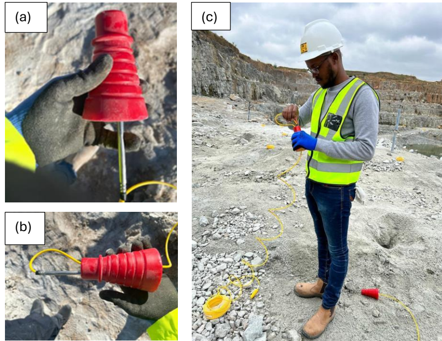
Figure 3.4: Booster-detonator with the insertion of the detonator done on the front side (a) and backside (b) of the booster; (c) Locking detonator in position before inserting in the blasthole (Source: Picture taken on site)
