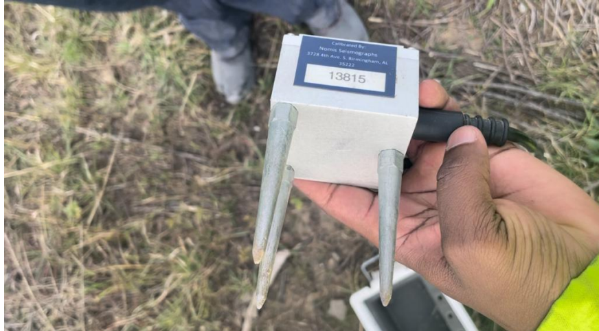
Figure 3.23: Geophone spikes (Source: Photo taken on site)
