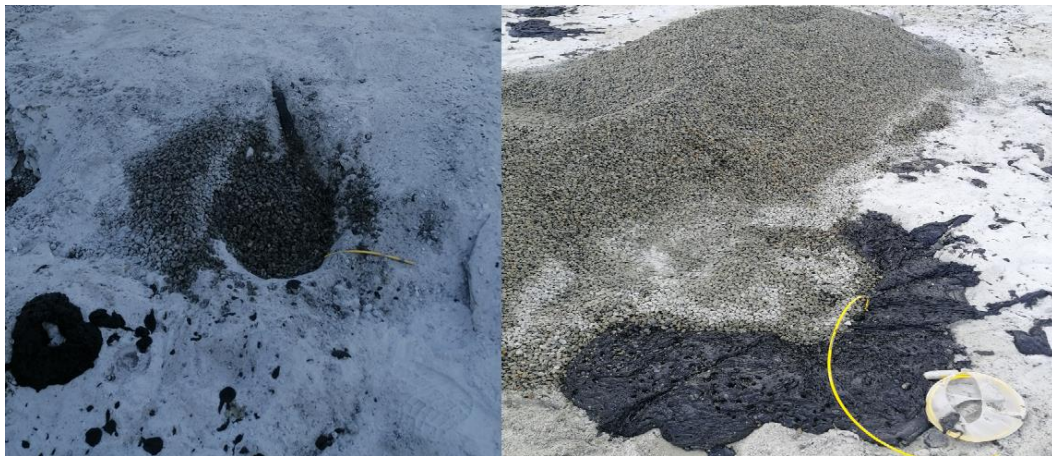
Figure 3.15: Blast-hole stemmed to the collar level (Source: Photo taken on site)
