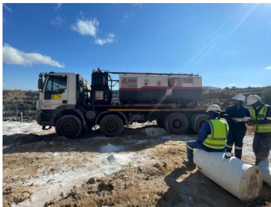
Figure 3.6: Explosive truck (Source: Picture taken on site)
