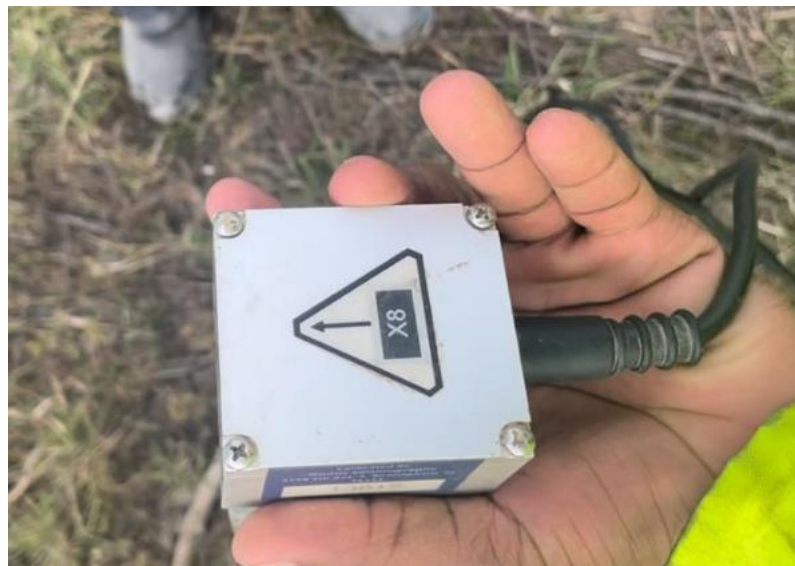
Figure 3.24: Geophone transducer arrow (Source: Photo taken on site)
