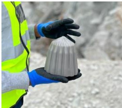
Figure 3.11: Varistem® plugs of diameter 102 mm (Source: Photo taken on site)
