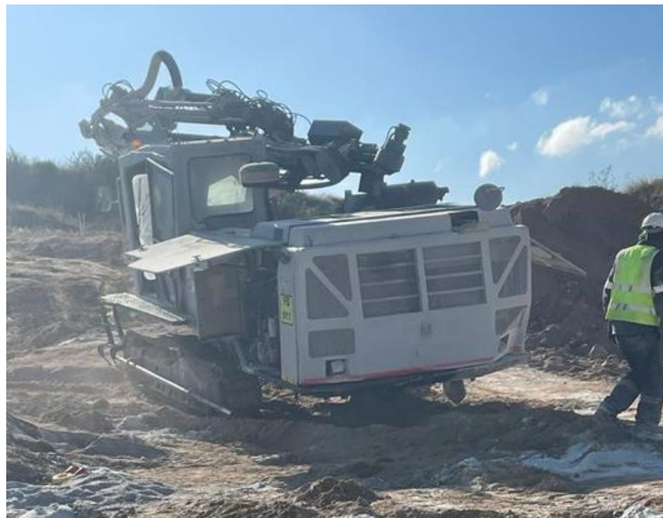
Figure 3.2: Surface drill rig (Source: Photo taken on site)
