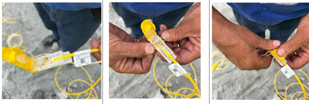
Figure 3.19: How to connect the detonator connector clip to surface wire – (Left) Opening the connector clip; (Centre) Connecting the wire; (Right) Closing the connector clip (Source: Photo taken on site)
