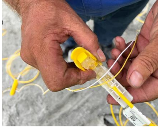
Figure 3.5: Colour-coded connector clip (Source: Picture taken on site)
