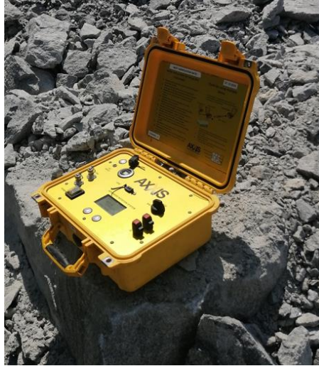
Figure 3.20: AXXIS Titanium Blasting box (Source: Photo taken on site)
