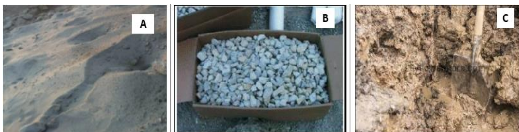
Figure 2.3. Different types of materials that can be used for stemming: A – Drilling cutting stemming materials; B – Crushed aggregate rock; and C – Clay stemming material (Reddy et al., 2020)
