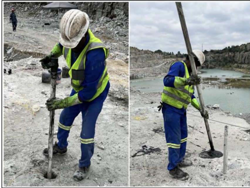
Figure 3.22: Excessive emulsion sucked out of the blastholes using a PVC pipe (Source: Author's own picture)
