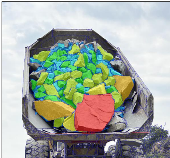
Figure 3.35: Image-based monitoring of the truck feed fragmentation at the quarry (Source: Author's own picture)
