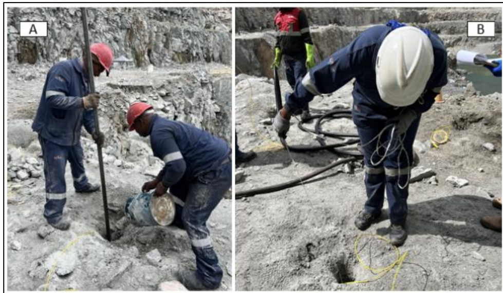
Figure 3.24: Stemming process – (A) Tamping and stemming; (B) Taking measurements after gassing using a tape measure (Source: Author's own picture)
