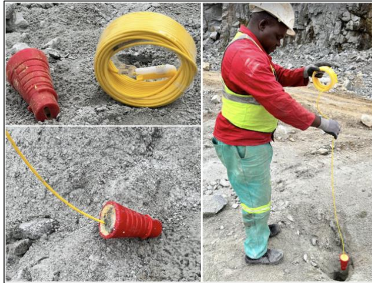
Figure 3.20: Priming of a blast hole – The typical red C-400 booster used in the various blast tests is shown on the top right with the yellow wire holding the AXXIS GII detonator (Source: Author's own picture)
