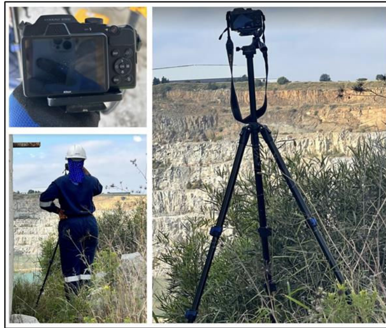
Figure 3.27: Configuration and setting up of the blasting camera (Source: Author's own picture)
