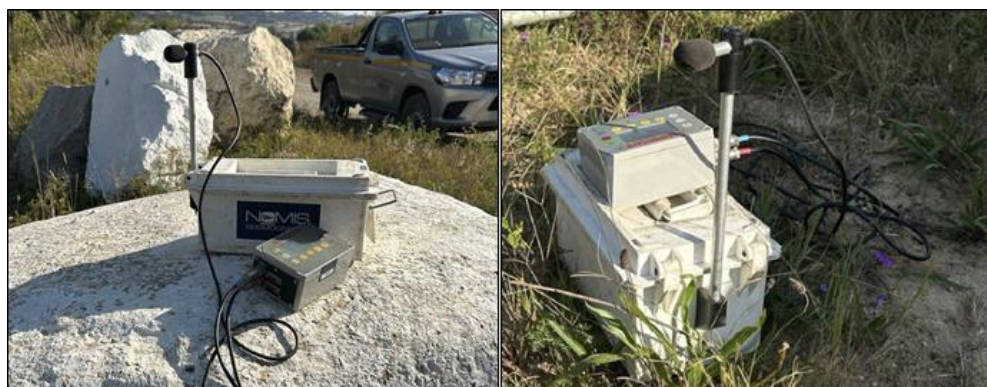
Figure 3.30: The two Nomis Mini Supergraph seismographs used on site to monitor ground vibrations and airblast (Source: Author's own picture)
