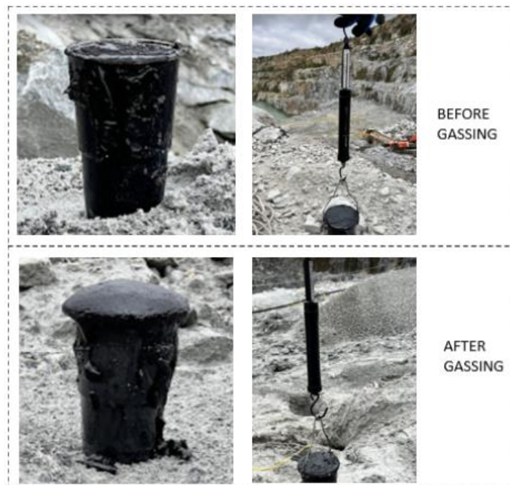
Figure 3.23: Weighing of the standard cup of emulsion before and after gassing (Source: Author's own picture)
