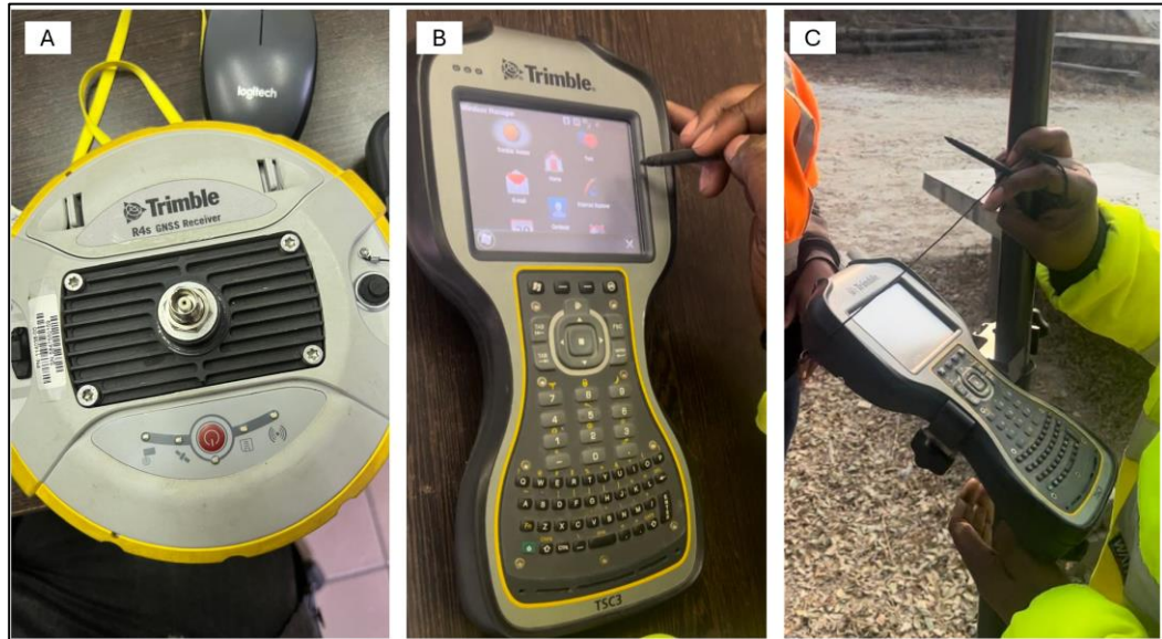
Figure 3.5: (A) Trimble R4s Global Navigation Satellite System; (B) Trimble TSC3 controller; and (C) TSC3 and R4s GNSS mounted on a 2-m antenna (Source: Author's own picture)
