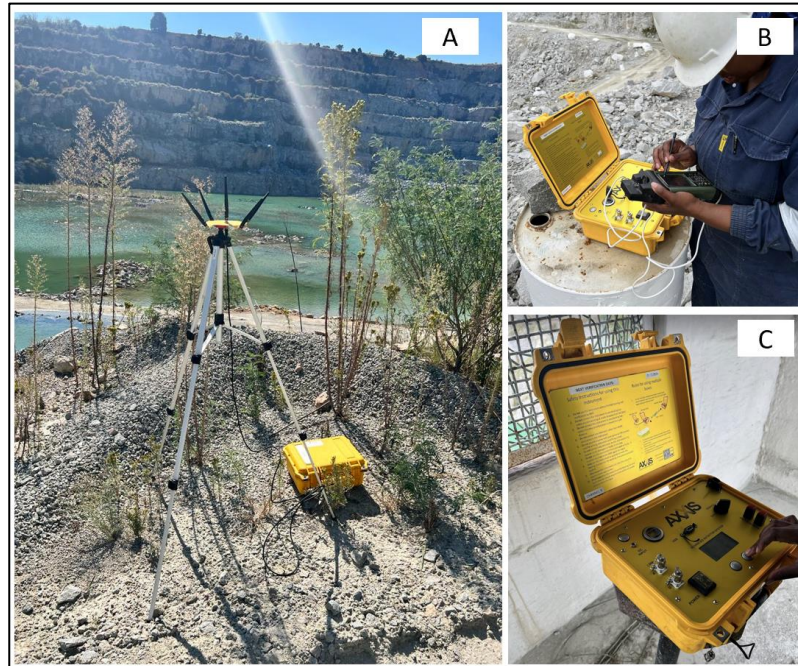
Figure 3.26: (A) Remote slave box; (B) Blaster verifying the blast connections; and (C) Remote master initiating box (Source: Author's own picture)
